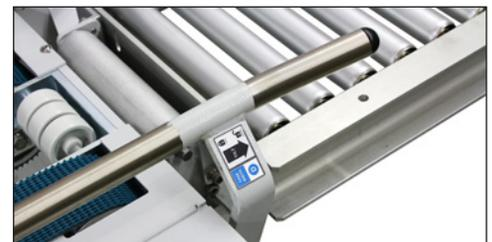
*Quick size change with top wheel and tilting guide rails*
